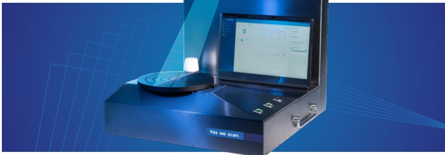
Our QUALIMETER was developed for random quality control of printed circuit boards, plastic parts, metallic components and ceramic components. The focus was placed on optimum detection of the object and therefore maximum precision of the evaluated parameters.
